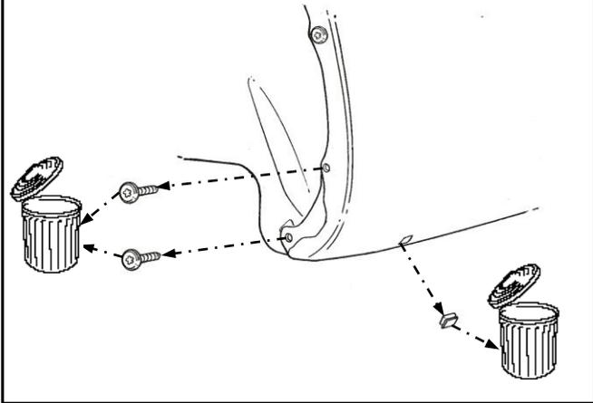
2) Remove existing screws -15mm and hole plug and discard.
